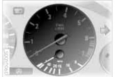
Indicates the current fuel consumption in mpg (in liters/100 km on Canadian vehicles). This allows you to see whether your current driving style is conducive to fuel economy with minimum exhaust emissions.
