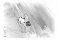
5 Then connect the negative terminals. Attach the cable to either the support vehicle's negative battery terminal (-), or to a suitable ground on its engine or bodywork. Then connect the other end of the cable to a ground on the engine or on the bodywork of the vehicle that is to be started. There is a special nut for this on the left side panel of your BMW. Refer to the arrow in the illustration.
