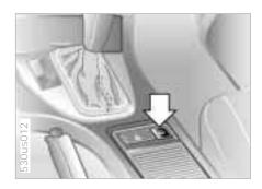
You can operate the central locking system with this button (arrow) when the driver's door is closed. The doors and tailgate/liftgate are unlocked or locked only. However, the antitheft alarm system is not activated. Also, the fuel filler door remains unlocked to allow refueling.
