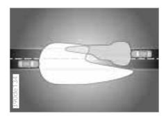
Xenon lamps illuminate the side and front areas of the vehicle with significantly more brightness and uniformity than traditional halogen lamps.
