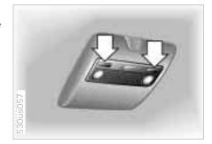
Reading lamps are provided in the front and rear\* near the interior lamp. They can be switched on and off with the button (arrows) next to each lamp.
