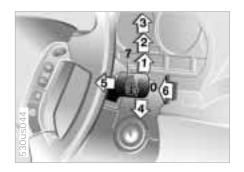
You can leave the lever permanently in position 1. It is then only necessary to activate the rain sensor from ignition key position 1 and up. To do this,
