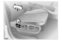
3 Backrest angle Pull the lever and apply weight to or remove weight from the backrest as required
