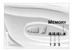
You can store and call up three different seat, exterior mirror and steering wheel positions. The illustration shows the buttons on the seat for making these position adjustments.
