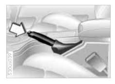
The parking brake is primarily designed to prevent the vehicle from rolling while parked. It operates against the rear wheels.
