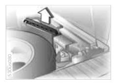
4 Remove the support rod from the bracket.
