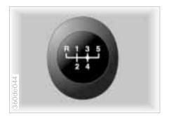
Press the clutch pedal all the way down each time you shift, pressing the manual-shift gear lever into its proper end position.
