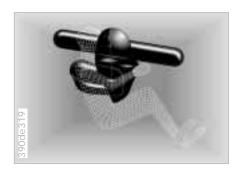
Deceleration sensors continuously monitor the physical forces acting upon the vehicle. If, as the result of a frontal impact, vehicle deceleration is reached at which the protection of the safety belts alone is no longer adequate, the gas generators of the driver-side and passenger-side airbags are ignited simultaneously. However, the passenger-side airbag is only triggered if an additional sensor has recognized that the passenger seat is occupied.
