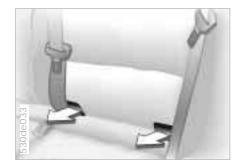
LATCH child seat attachment\* Remove cover panel by pulling it off toward the front. Simply put it back on to reattach it.
