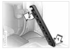
6 Insert the support rod in the tailgate lock and press down until it engages (arrow 1); then lock hook of rod in striker (arrow 2).
