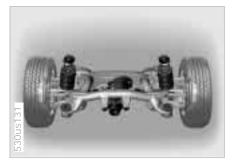
This axle is based on the same multilink principle as that in 7 Series vehicles. The axle's kinematics and elastic kinematics are critical for wheel control – a significant prerequisite for achieving the objective of exceptional onroad handling characteristics with this vehicle concept.
