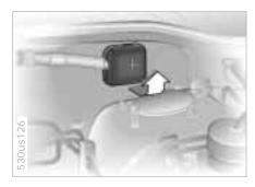
4 Start by connecting the jumper cable from the positive terminal of the support vehicle to the positive terminal connector located in your BMW's engine compartment The cover of the auxiliary terminal for jump starting is marked with a "+" sign (refer to the illustration). To remove the cover, tip up the cap (arrow). The illustration shows the auxiliary terminal for jump starting on the BMW X5 4.4i. For the BMW X5 3.0i: refer to "Engine compartment" on page 152.
