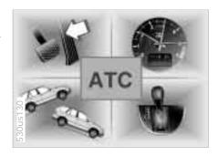
On vehicles with an automatic transmission, Adaptive Transmission Control (ATC) uses a number of factors to calculate the gear which provides the maximum efficiency. In this process, the system monitors your personal driving style, the driving situation, the condition of the road, and the traffic conditions.
