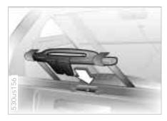
3 Hook both buckles into the latch of the tailgate (arrow); the tailgate is released.
