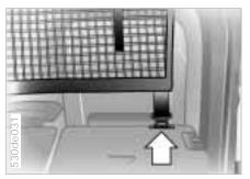
7 When the rear backrests are folded over, you can open the Velcro® strips, completely unroll the partition net, insert it in the front brackets on the roof and attach the three hooks into the eyes.
