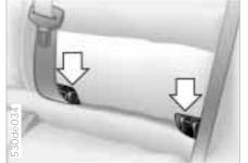
The illustration shows the mounts for a LATCH child-restraint system in the left rear seat.
