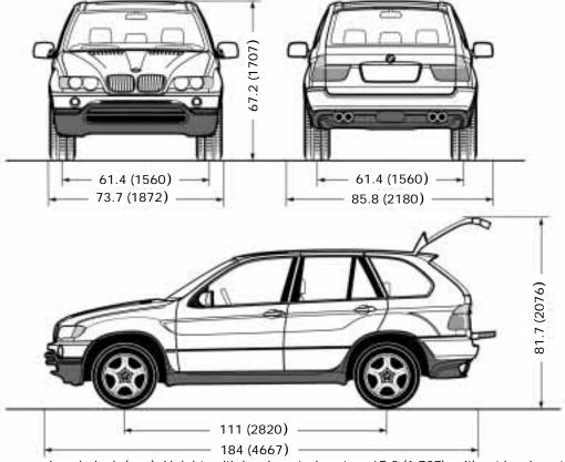
All dimensions are given in inch (mm). Height: with level control system 67.2 (1,707); without level control system: 67.5 (1,715). Height with roof-mounted luggage rack: with level control system 68.5 (1,740); without level control system: 68.8 (1,748). Track width X5 3.0i: 62 (1,576). Min. turning circle dia.: 39.7 ft (12.1 meters)
